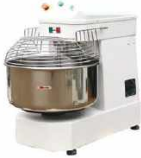
Spiral Mixer - 20 Litres (Double Speed) Dimension: 690 x 380 x 730(mm) Raw Flour : 8 Kgs. Power : 1.1 kw, 220V
